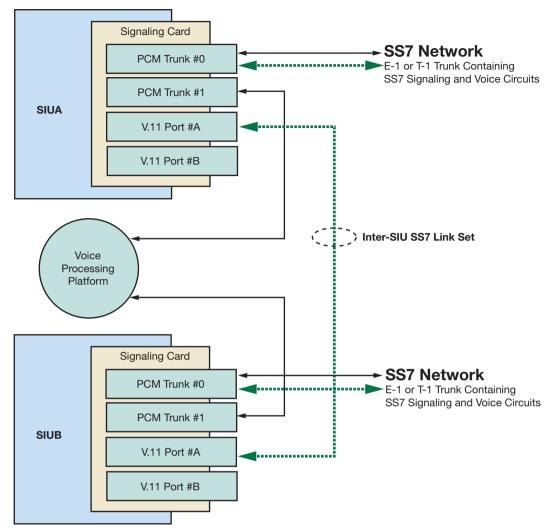
Figure 18. Inter-SIU Link Set over V.11
